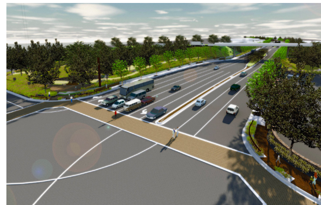
FIGURE 3: Vehicular surface represented by Road Object (Image courtesy of Pacific Coast Land Design)
